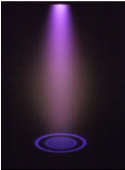
Figure 4: DC driven air glow discharge in a pin-water geometry with self-organization at the surface of the water anode electrode. Reproduced with permission from [56]. Table 1: Typical plasma properties for four often used discharges: pulsed direct discharge in liquid, DC air glow discharge with a water electrode, pulsed plasma jet (non-touching) and filamentary dielectric barrier discharge (DBD). These values are estimates as a guide to typical plasma conditions.
