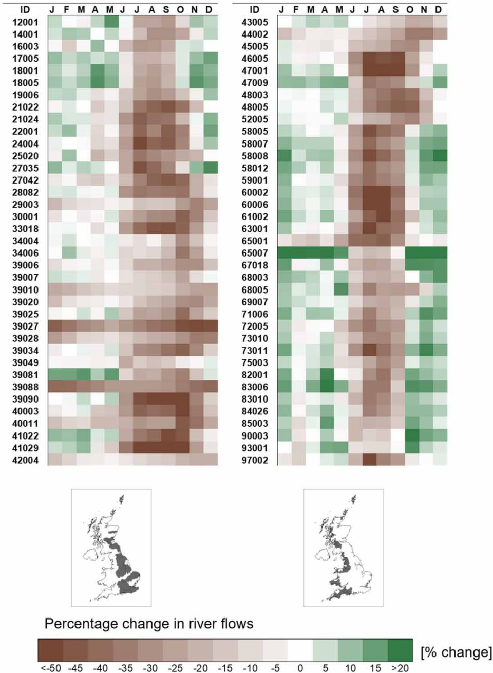
Figure 3 | Monthly percentage changes in river flows at the gauging station near RoR schemes. The baseline flows are the flows simulated using the GR6J hydrological model for the period 1980–2009. The near future flows are the mean for all the RCM simulated flows for the period 2030–2059. The maps below show the highlighted in grey the catchments where the gauges are in each column. Furthermore, the ID is equivalent to the gauge number, which is based on the NRFA system, consisting of the hydrometric area number, followed by three further digits (e.g., the IDs 21022 and 21024 correspond to hydrometric area 21, also known as the Tweed catchment). The legend refers to percentage change in mean monthly flows in the future from the baseline.
