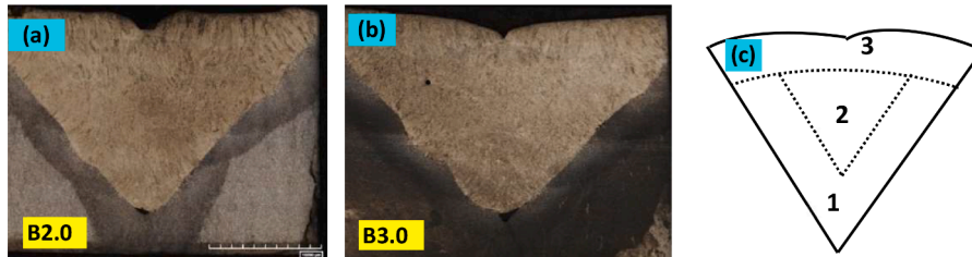
Fig. 15. (a & b) The macrostructures of LTT1 and LTT2 weld metals, (c) the schematic of the areas of microstructural examination.
