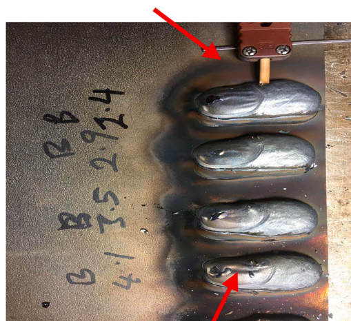
Fig. 5. Use of R-type thermocouple to measure phase transformation temperature.
