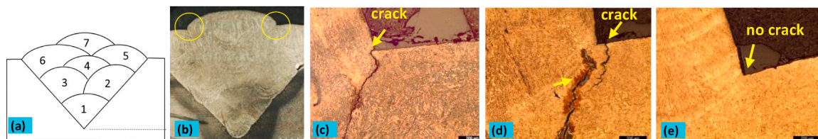
Fig. 3. Weld metals: (a) schematic of 7-pass weld, (b) 7-pass weldment showing toe or notch area examined, (c & d) typical cracking observed in the LTT alloy, (e) LTT alloy composition with no cracking.
