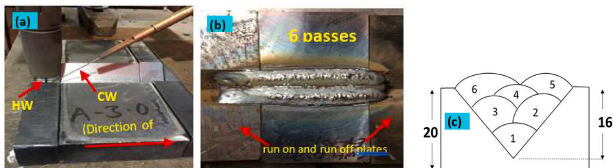
Fig. 2. (a) Welding set up: (b) 6-pass welded sample, (c) schematic of the 6-pass bead sequence.
