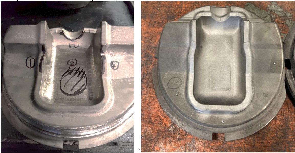
Figure 2: Die at EOL with areas of wear marked (left) and after remanufacturing (right)
