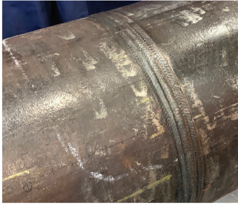
Figure 6. The 325 mm outer diameter mild steel pipe used for RGB-D brightness limitations experiment.
