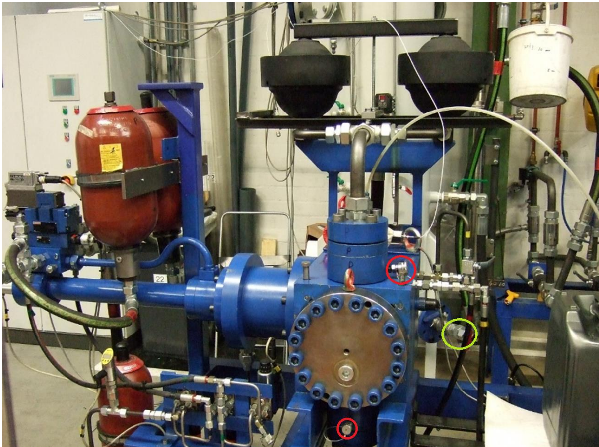
472 473 Figure 5 – Test rig for single chamber pump, where in red circle are highlight two piezo resistance sensors (at the suction 474 and the discharge valves) and in green the piezoelectric sensor for the chamber pressure value.
