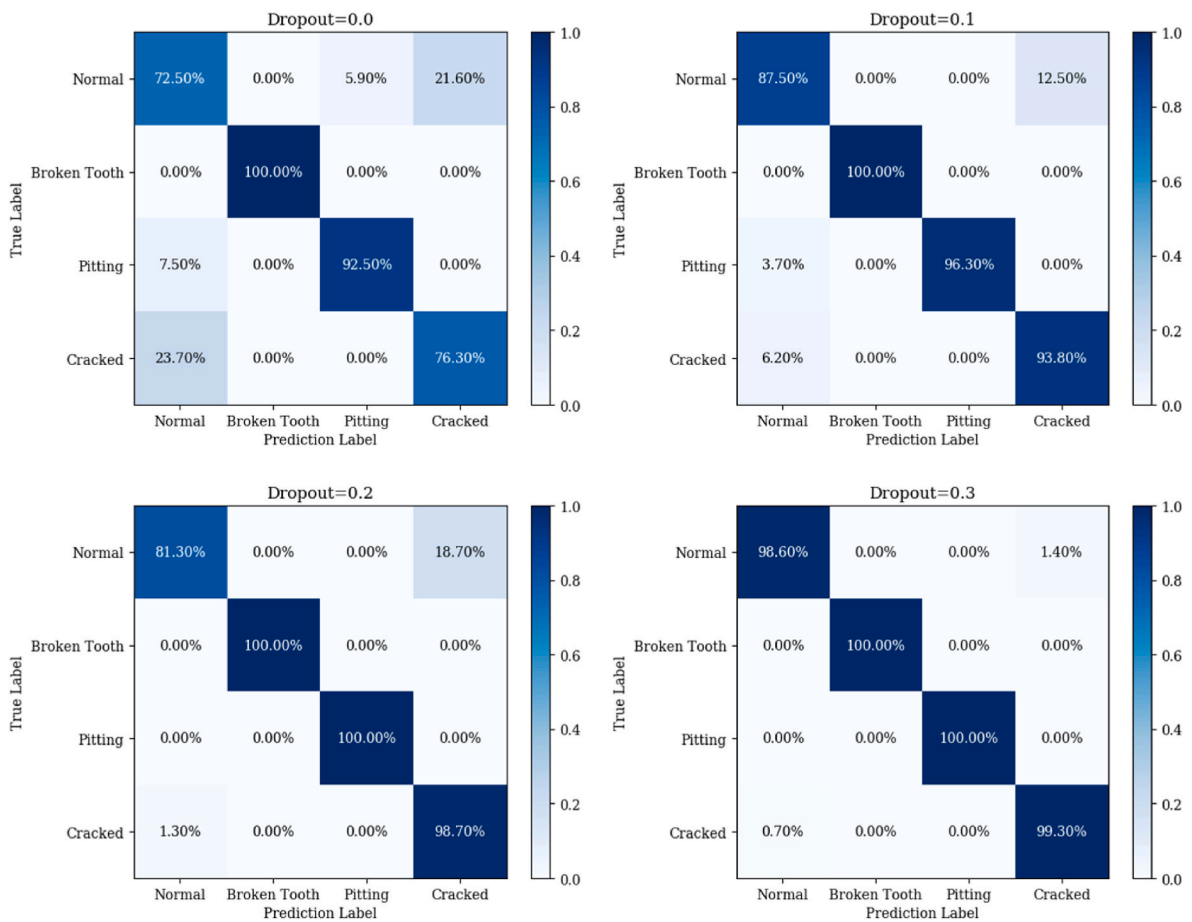
Fig. 12. Confusion matrices of CNN-LSTM on the simulation dataset with different Dropout ratios.
