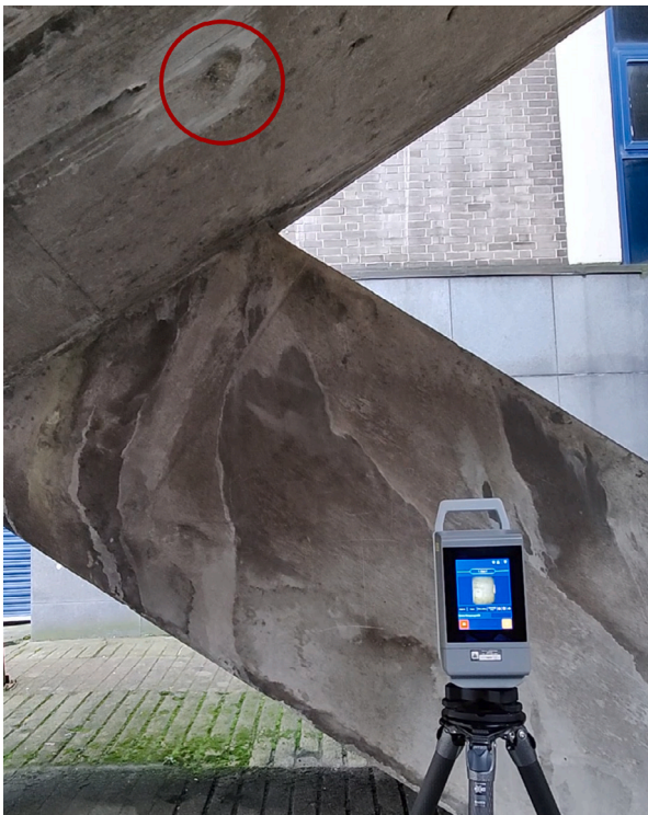
Fig. 6. Trimble X12 laser scanner data acquisition on field trial sample. The red circle highlights the spalling region.
