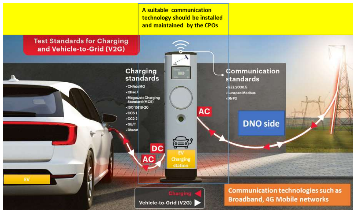
Figure 3 High level diagram shows how the EV communicate with the power grid
