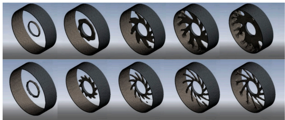
Figure 7. Structural optimisation process using generative design techniques [14].
