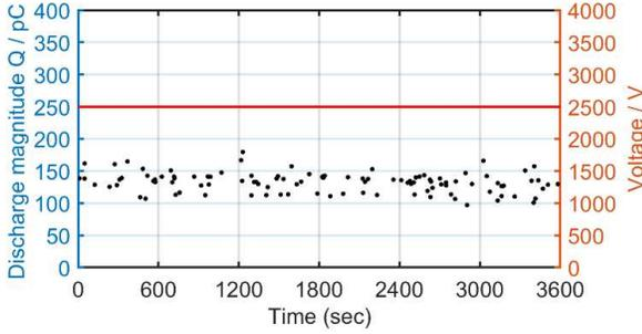
Fig. 4. Needle-plane discharge pattern under DC at the PDIV
