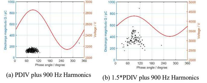
Fig. 5. The needle-plane discharge pattern under (a) the PDIV or (b) 1.5 times the PDIV in DC superimposed with 900 Hz harmonics.
