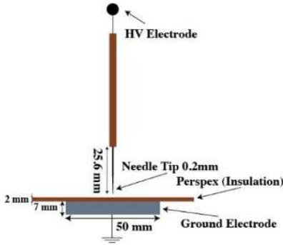
Fig. 1. Needle-plane test cell schematic
