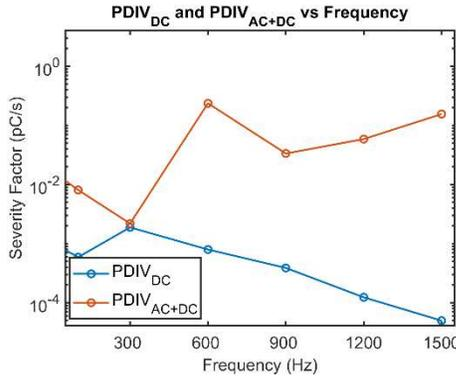
Fig. 6. SFs (pC/sec) of PDs in the 1<sup>st</sup> hour under the pure DC PDIV and in the subsequent hour with the superimposing of harmonics at different frequencies.
