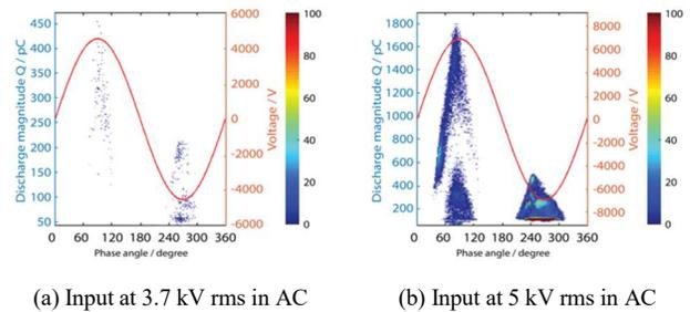
Fig. 3. Needle-plane corona discharge patterns under (a) the PDIV of 3.7 kV rms in AC and (b) 5 kV rms in AC. (The discharge intensity is presented by colormaps).
