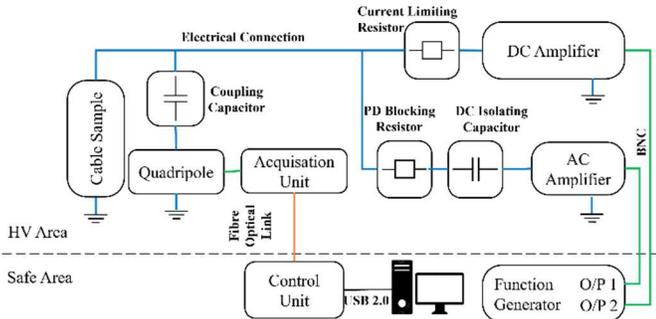
Fig. 2. Block diagram of the experimental setup
