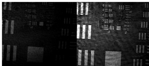
Fig. 2. SNR increase in the image of the USAF target mounted behind a scattering layer obtained with high-throughput FD-FF-OCT system (right) compared to a standard FD-FF-OCT system (left).
