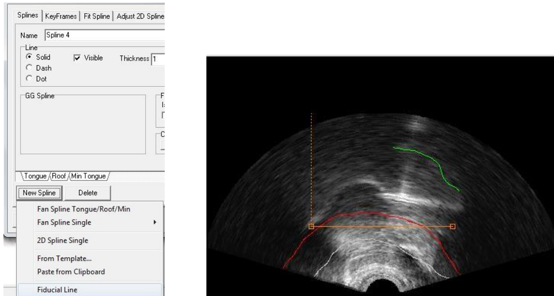
Figure 31: Adding a fiducial line to the ultrasound pane to represent the bite-plane trace.
