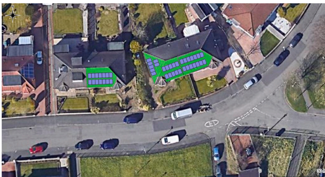
Fig. 5. Example of script identifying south-facing rooftops represented by green polygons, and its area passed to the in-built solar PV model with PV panels represented by blue polygons.
