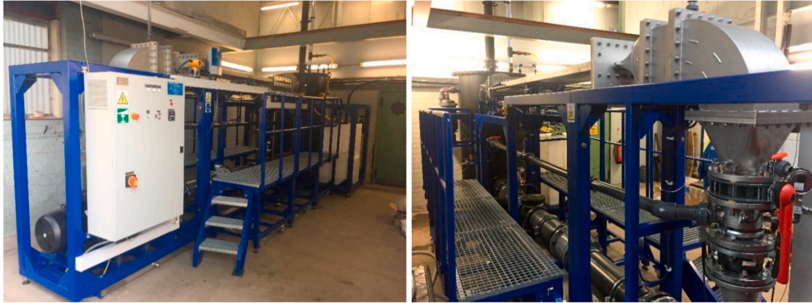
Fig. 2. A general view of the FTFC, left: control unit and visual access side of the FTFC, right: pump outlet and contraction pressure tap side of the FTFC.
