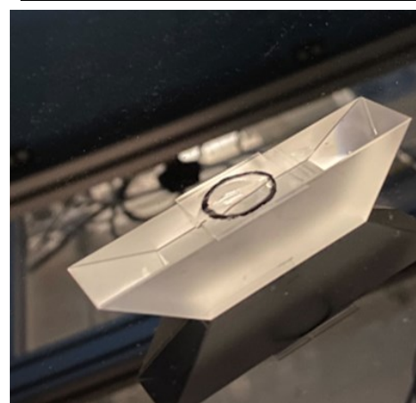
Left centre: prism preparation for nanodiamond imaging with adhering to prism. Consists of two coverslips (ND mount on the top) which are sealed and mounted on oil to the prism.
