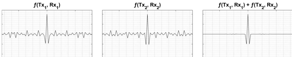
Fig. 1. Demonstration of sidelobe suppression by the sum of two complementary Golay functions, resulting in a single main lobe
