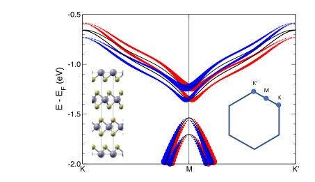
**Figure 5.** Spin–orbit splitting of the valence bands in 3R-MoS<sub>2</sub>: black lines show the band structure without spin–orbit coupling (SOC), red/blue dots indicate the spin polarization perpendicular to the layers (up/down) of the bands with SOC included. Insets show the structure (grey/yellow spheres: Mo/S) and the Brillouin zone.
