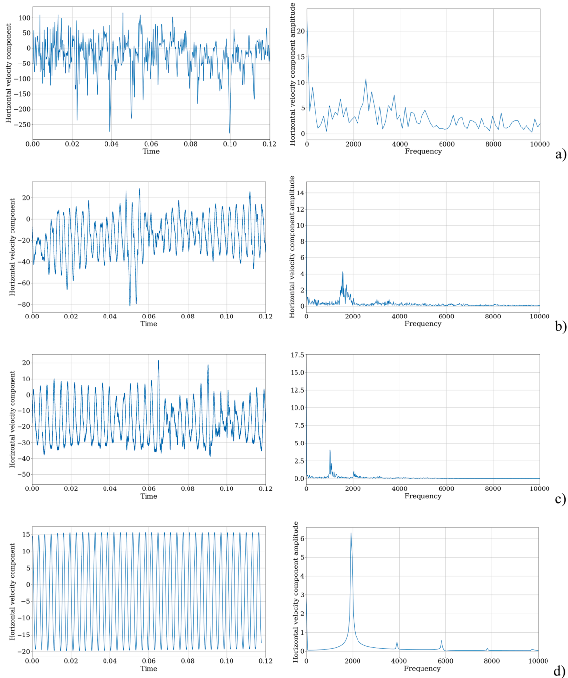
Fig. 19. 3D numerical results: Horizontal velocity component as a function of time (left) and related frequency spectrum (right) at x = 1/2, y = 1/2, z = 5/8 and T_{\text{cold}}=60\text{ }^{\circ}\text{C} ( Ra=8.74 \times 10^7 ): a) Bi=2.1 , b) Bi=4.2 , c) Bi=6.3 , d) Bi=10.56 . Starting from a situation with chaotic behavior, the flow undergoes a gradual stabilization until a perfectly time-periodic state is recovered.
