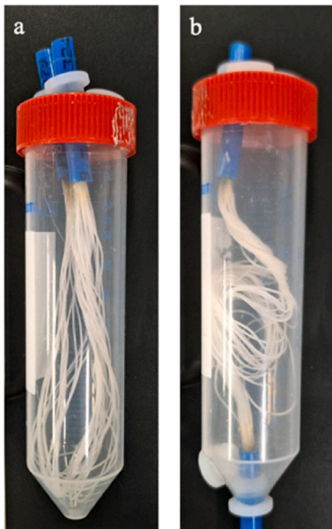
Fig. 5. Different configurations of a membrane module with 20 cm long hollow fiber membranes in a modified centrifuge tube a) U-shaped configuration with both ends on the lid, b) I-shaped configuration with ends at opposite sides.
