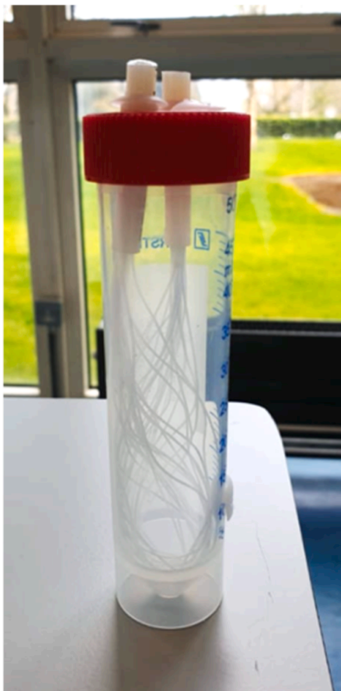
Fig. 2. Modified 50 ml centrifuge tube with silicone grommets to connect membrane bundles and tubing.
