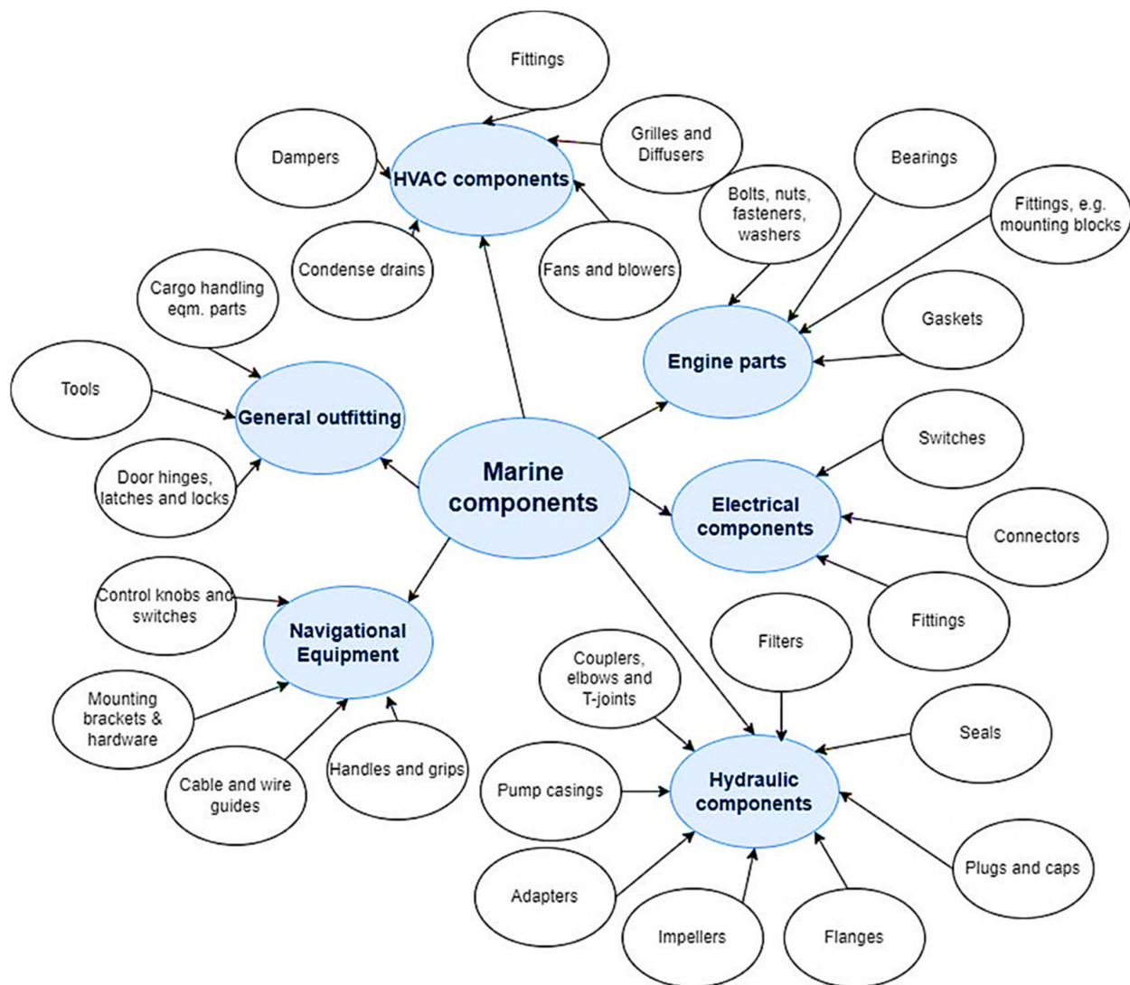
Figure 2. Systems-based breakdown of maritime auxiliary components potentially suitable for additive manufacturing.
