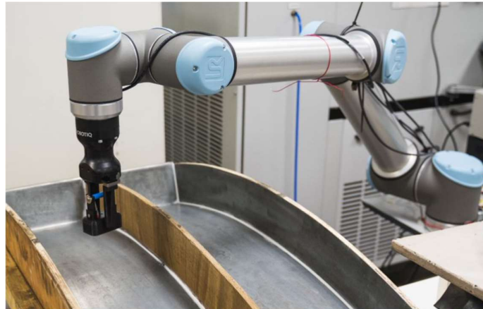
Figure 2. Robotic PnP of magnetic box with a 6-axis robotic arm
