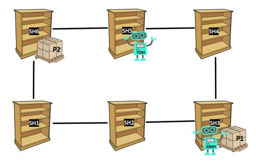
Figure 2: Diagram of the warehouse delivery system domain. SH<sub>-</sub> are shelves, P<sub>-</sub> are packages, and Tom and Jerry are robots responsible for delivering the packages to their correct shelves. The black lines indicate the paths the robots can traverse the shelves.
