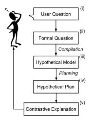
Figure 1: The five-stage iterative process for generating a contrastive explanation from a user question. The hypothetical model is created by compiling the formal question into the planning model (in PDDL 2.1), a planner is used to solve the model and produce a hypothetical plan.
