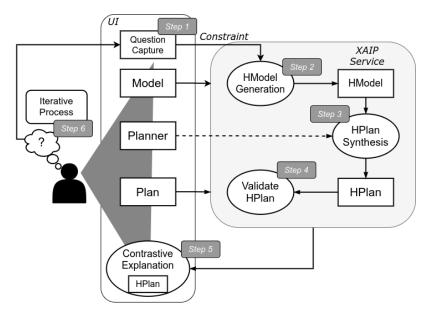
Figure 20: Proposed approach for Explainable Planning as a service. Starting from step 1, a user asks a contrastive question about a plan for a model produced from their planner. The XAIP Service first generates the HModel from the user question and uses the same planner to produce an HPlan. The HPlan is then validated and used to generate a contrastive explanation. The process can then be repeated from step 1.
