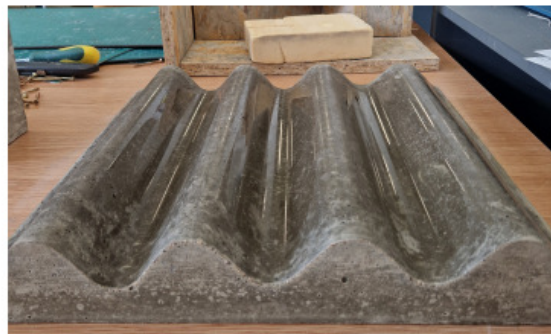
Step 5: Remove shutter-work
