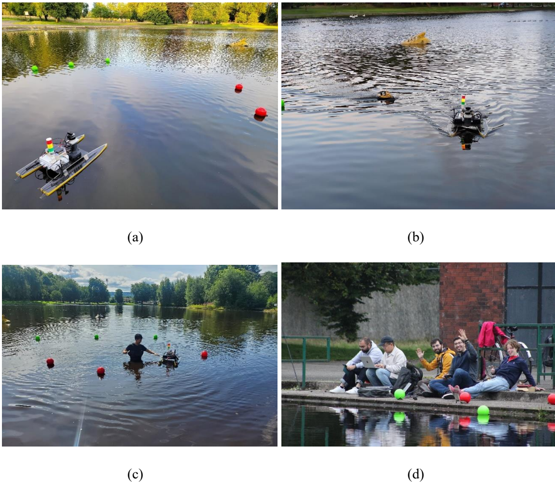
Figure 23 Outdoor tests on (a) buoy gate passing (b) obstacle avoidance (c) recovering boat during testing (d) students debugging at the pond.
