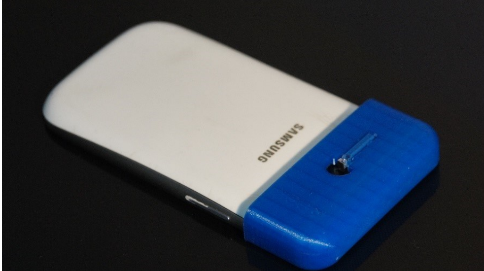
Fig 4. Peek Vision Smartphone-based retinal Imager
