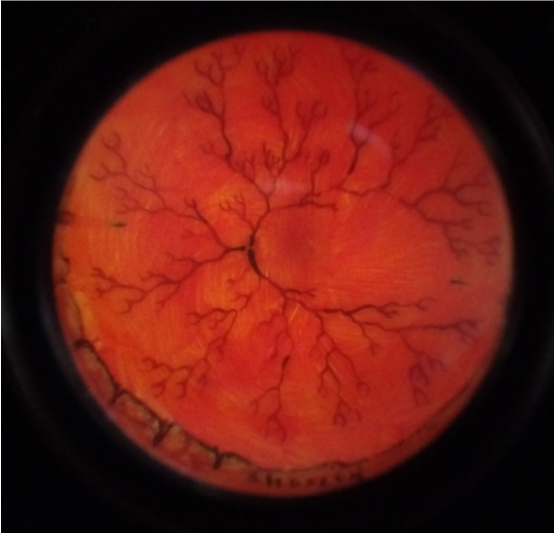
Fig 10. Images taken with the self-operated retinal imager on a translucent eye phantom A) without the illumination system B) with the illumination system
