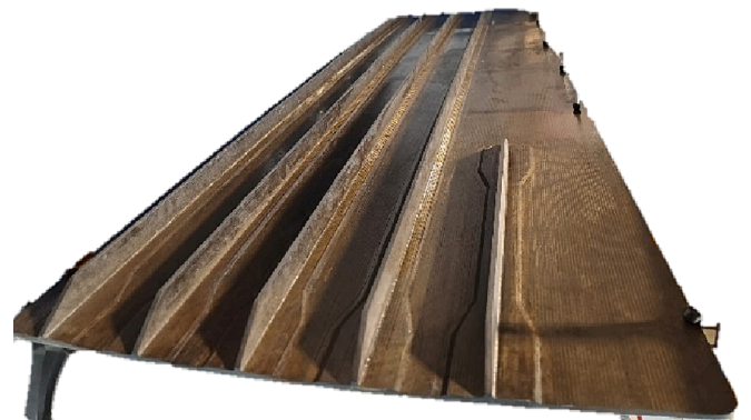
Fig. 7. Wing cover component with complex geometry and varying thickness.
