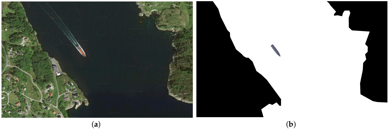
Figure 5. (a) Satellite image of a navigational area captured using Google Maps. (b) 2D occupancy grid map of the navigational area.
