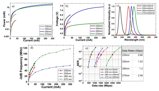
Figure 1 a) The LI b) IV c) spectra d) modulation bandwidth e) BER vs data rate for the 235nm, 255nm, 265nm and 275nm LEDs.
