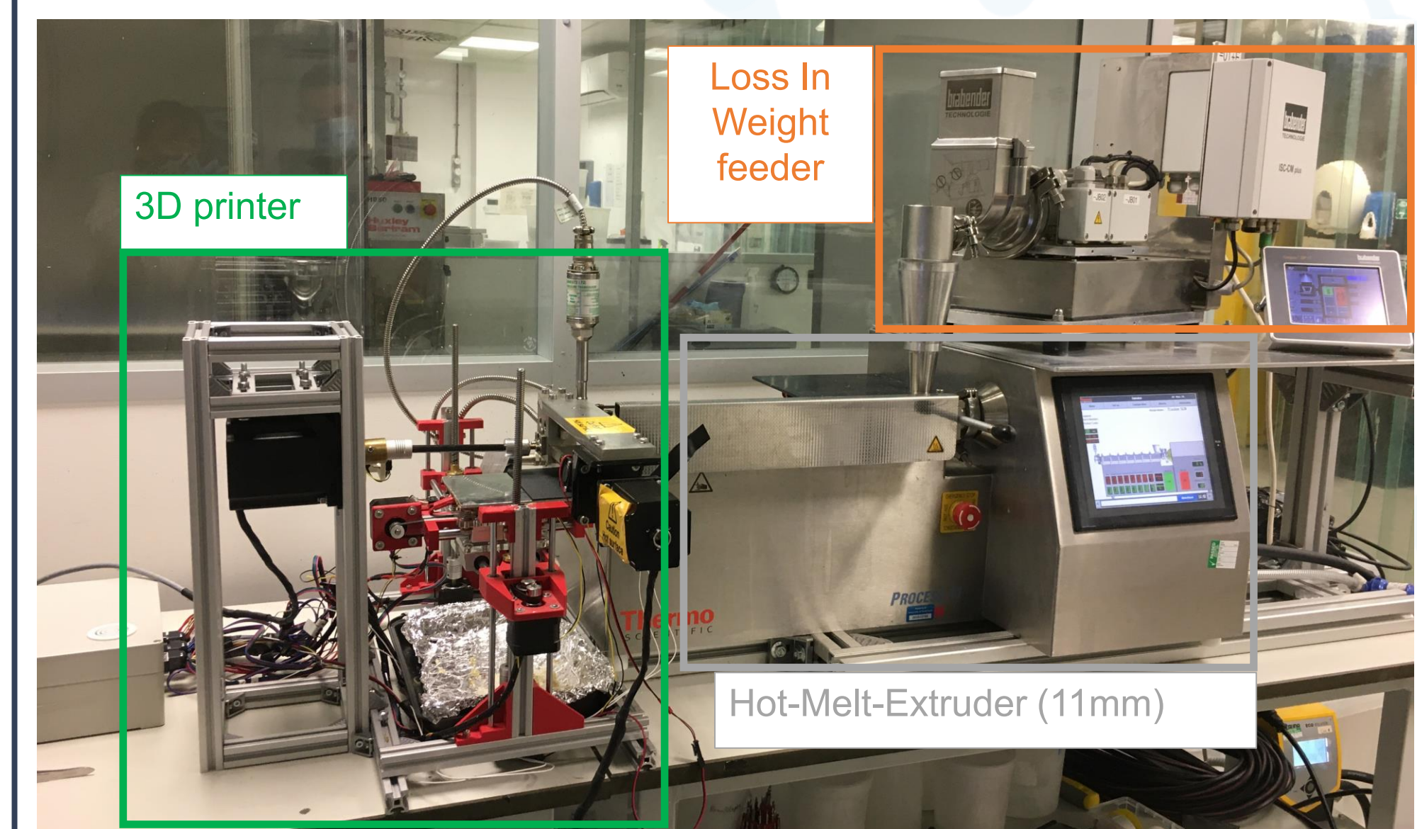
Figure 4: Novel filament free Hot-Melt-Extrusion 3D printer: Loss in Weight Feeder, HME (Process 11, Thermo Fisher) and 3D printer unit.
