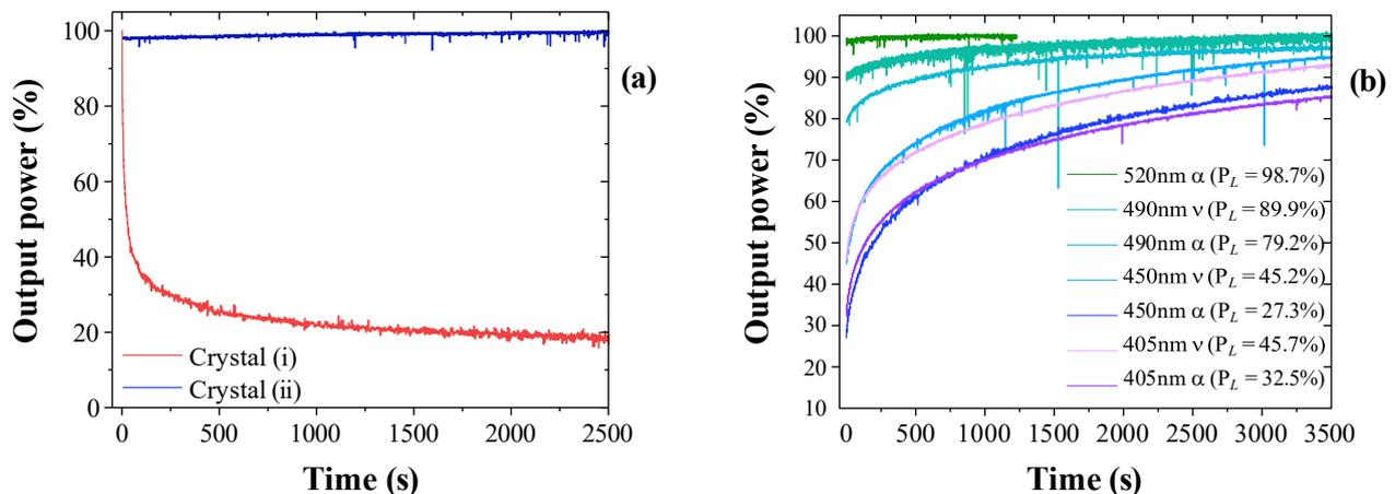
Figure 1: (a) Normalised resonator output power traces under  $\pi$ -polarised 450nm pumping for crystals (i) and (ii), and (b) resonator output during  $\pi$ -polarised 520nm annealing from the  $P_L$  state, annotated with the wavelength and polarisation of loss-induction preceding the annealing, and the starting power as a percentage of the final power.
