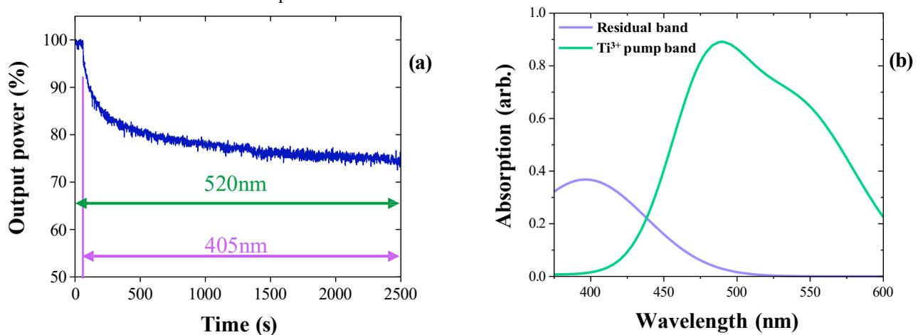
Figure (2): (a) Normalised output power for crystal (ii) under  $\pi$ -polarised 520nm pumping at the point when co-pumping with  $\sigma$ -polarised 405nm diode is initiated, (b) schematic absorption spectrum of Ti:sapphire in  $\pi$ -pol, delineating the residual and pump band contributions, noting the region of overlap between 400-500nm.
