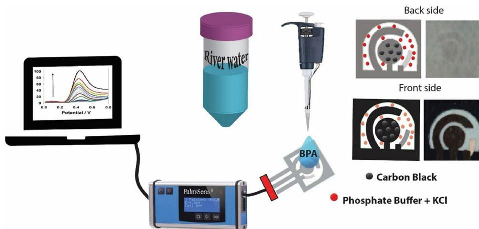
identify the presence of BPA in river water. The described paper-based electrochemical sensor was inexpensive, portable, and easy to use, with sample flow achieved without the use of external pumps.
