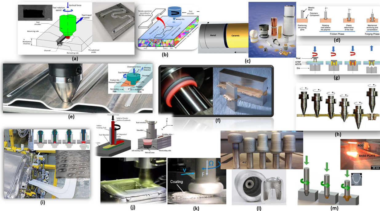
Figure 1. Popular friction-based manufacturing processes: (a) Friction stir channeling [43, 44] ; (b) Friction stir processing [92] ; (c) Friction brazing [93, 94] ; (d) Friction riveting [95] ; (e) Friction stir welding [96, 97] ; (f) Friction welding [98, 99] ; (g) Friction self-piercing riveting [100] ; (h) Friction drilling [101] ; (i) Friction stir spot welding [102] ; (j) Friction stir additive manufacturing [103-105] ; (k) Friction surfacing [5] ; (l) Friction flash to tube [106] ; (m) Friction hydro pillar processing [107] .
