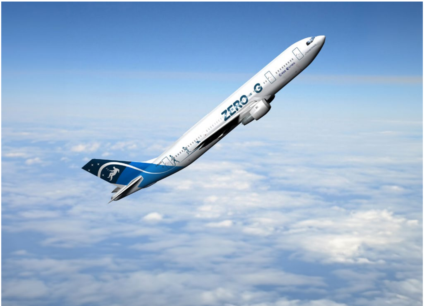
Figure xi. Refitted Airbus A310 aircraft for parabolic flights (Credit: Novespace & European Space Agency)
