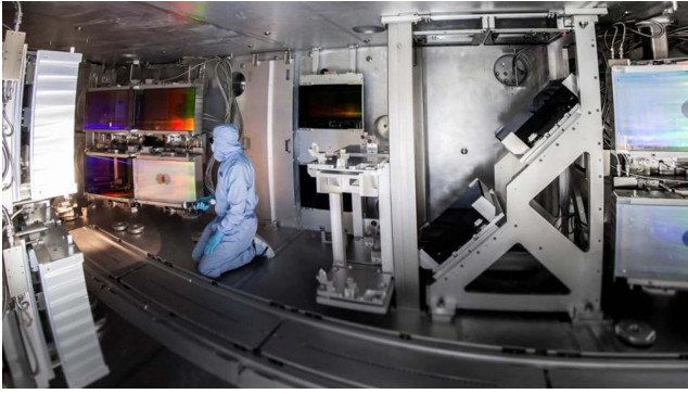
Figure 5. NIF ARC compressor gratings during final alignment (picture courtesy of LLNL).
