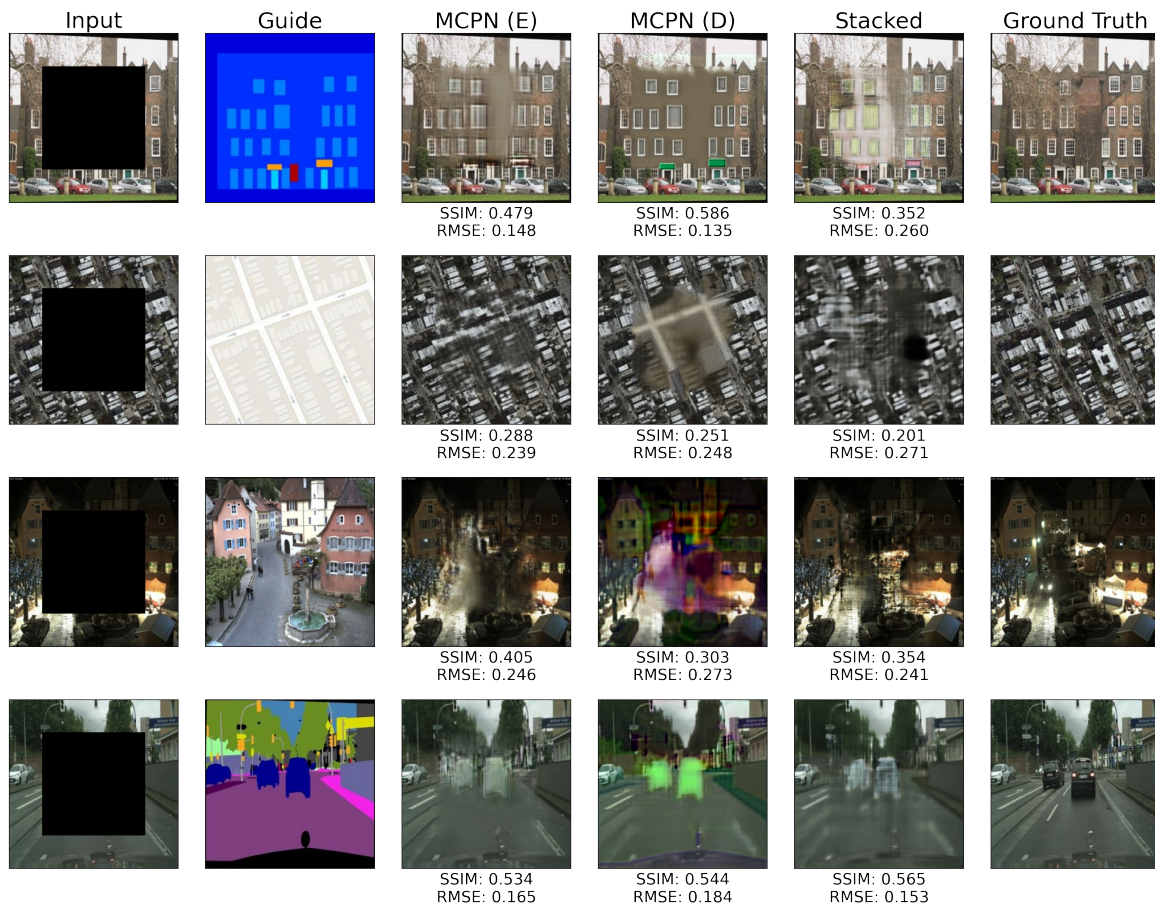
Figure 11. Example output for the three tested inpainting methods for each experiment dataset (from top to bottom: Facades, Map-to-Aerial, Night-to-Day, Cityscapes). The reported metric values correspond to the inpainted area only.
