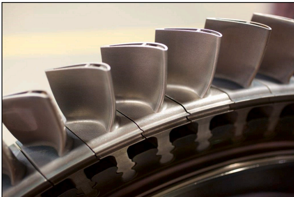
Fig. 9. Gas Turbine Blades made for Siemens by Material Solutions [23].
