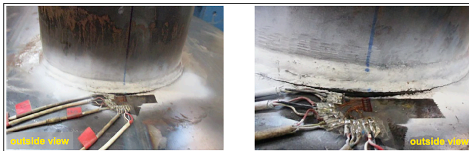
Fig. 21. Through-Thickness Fatigue crack development for WTJ-7 after 4060 at P = 90 kN [50].
