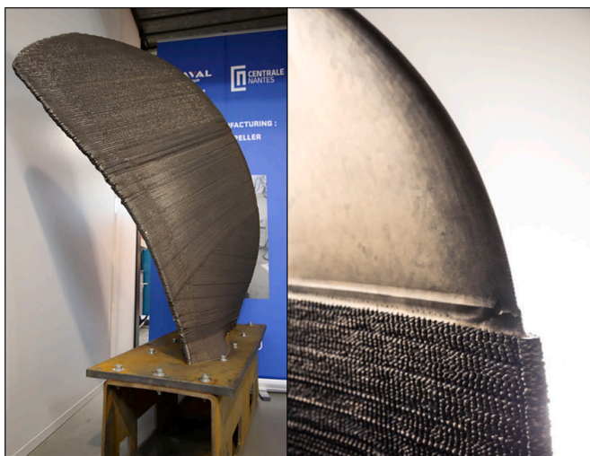
Fig. 10. Propeller Created via WAAM Manufactured by French Naval Group [24].
