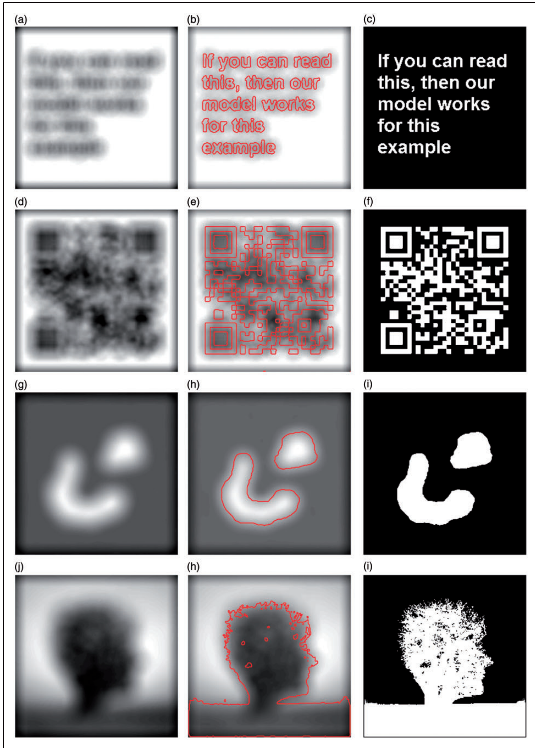
Figure 7. Result set 3. Illustration of the performance of the New l for (top-bottom) Im_1 , Im_4 , Im_2 and Im_6 corrupted by strong Gaussian blur. New l is capable of segmenting edges in these challenging cases which cannot be segmented by Mod 1 .
