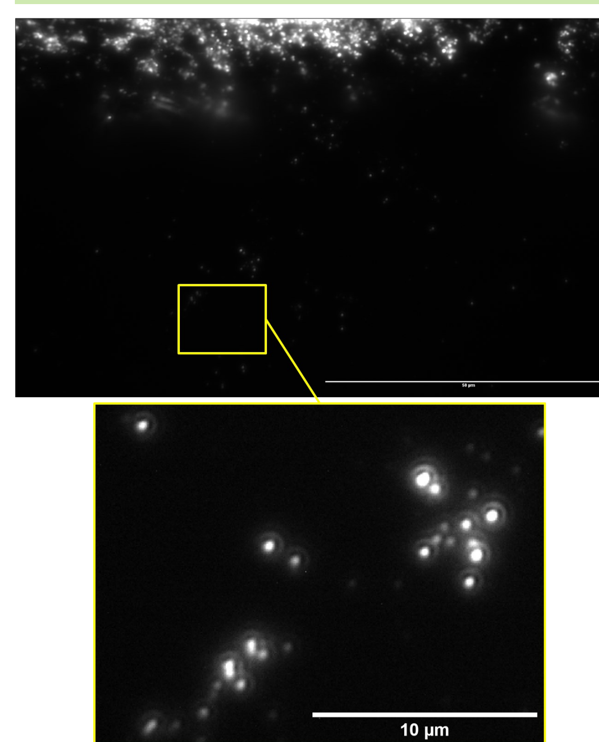
Top Left: 90nm FND in full field of view Bottom Left: FND zoomed in to show Airy rings. Right: Continuous wave frequency sweep 2.81-2.93GHz in steps of 5MHz.
