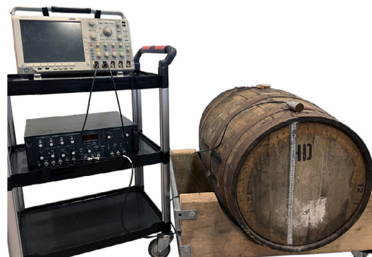
Fig. 9. Practical experiment setup for horizontal stored cask measurements.
