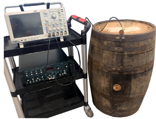
Fig. 12. Practical experiment setup for vertical stored cask measurements.
