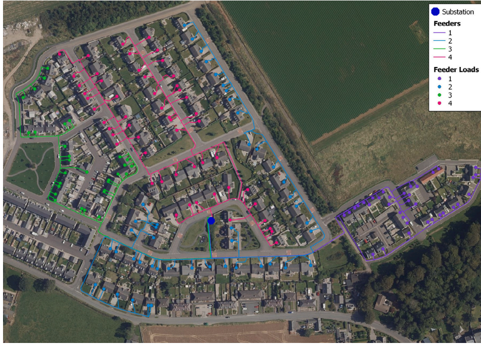
Fig. 7. Satellite visualisation of the low voltage distribution network under study using Bing Aerial showing which households are connected to which of the four network feeders in the area that are connected to the substation shown.
