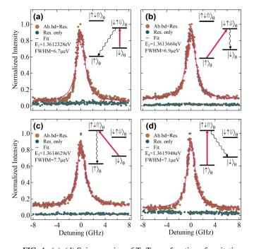
FIG. 4. (a)–(d) Spin pumping of  $T_1$ – $T_4$  as a function of excitation laser detuning under the oblique configuration. Emission intensity vs single photon counts shown with (i) randomization and (ii) no randomization applied. Solid line is Lorentzian best fit. Inset (top right) shows excitation and detection scheme for each.
