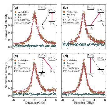
FIG. 5. (a)–(d) Spin pumping of  $T_1$ - $T_4$  as a function of excitation laser detuning under the Voigt configuration. Emission intensity vs single photon counts shown with (i) randomization and (ii) no randomization applied. Solid line is Lorentzian best fit. Inset (top right) shows excitation and detection scheme for each.
