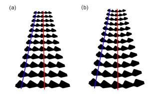
FIG. 9. (a) Example of a straight taper of 11 lines shrinking by a factor of 2 (5% per line). (b) Example of a rounded taper. The unit cells are now also rotated such that the lattice locally keeps its original shape. The traps along the two red lines are similar but the traps along the blue lines differ due to the different transformation.
