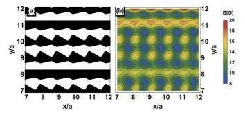
FIG. 6. (a) The same magnetic film pattern as Fig. 5. (b) The potential created by the film of (a) with the reversed external field:  $\mathbf{B}_{\rm ext} = (10, 9.0, 5.0 \times 10^{-2}) \, G$ . A three-rail ladder is created by the same structure as Fig. 5 with reversed external field to create wells above the other edge of the magnetic structures.
