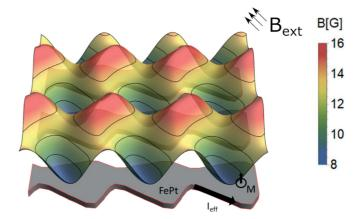
FIG. 1. Three-dimensional representation of the magnetic potential in arbitrary units above an out-of-plane magnetized patterned layer of FePt (gray). The potential is calculated at a height z=0.5a above the surface, with a the lattice constant. The external magnetic field  $\mathbf{B}_{\rm ext}$  was chosen such that a square trapping potential with equal barrier heights at z=0.5a is obtained:  $\mathbf{B}_{\rm ext}=(-10,-9.0,-5.0\times10^{-2})~G$ .
