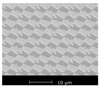
FIG. 4. SEM image of the honeycomb lattice with lattice spacing of 5  $\mu$ m. Lighter regions indicate magnetic material.
