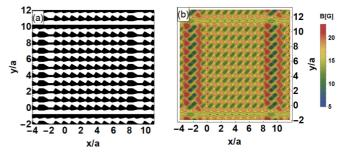
FIG. 7. (a) Magnetic film pattern with  $a=5~\mu m$  where horizontal and vertical barriers have been combined to isolate a plaquette of  $10\times 9$  sites. (b) The potential created by the film of (a) with the same external field as for a square lattice with periodic barriers:  $\boldsymbol{B}_{\rm ext} = (-10, -9.0, -5.0\times 10^{-2})~G$ .
