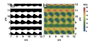
FIG. 5. (a) Magnetic film pattern with  $a=5 \mu m$  that can create a double-well series or two-rail ladder. The external field is here set to generate equal barriers between all ladder sites and is  $\boldsymbol{B}_{\rm ext} = (-10, -9.0, -5.0 \times 10^{-2}) \, G$ .
