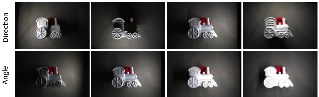
Figure 5: Example output images from the photometric stereo test rig with the train object. The top row shows the different lighting directions (images left to right): lighting from left, bottom, right, top.
