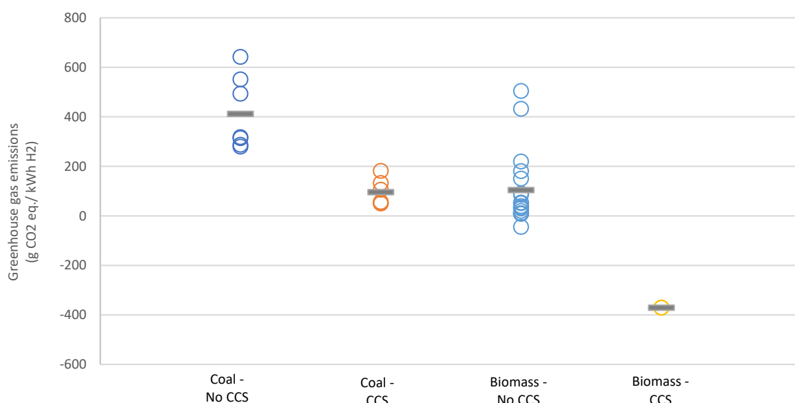
Figure 9. Greenhouse gas emission estimates of hydrogen from coal and biomass gasification. Grey bars represent the mean emission across the literature for each category.
