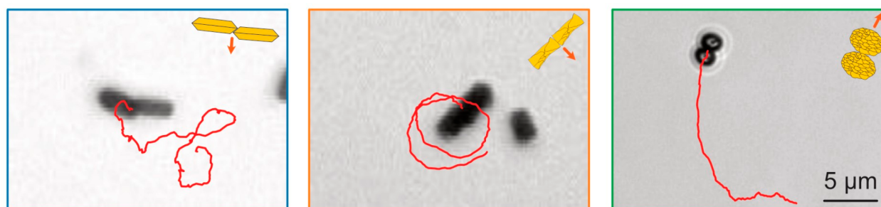
Figure 10. Light micrographs of assemblies of two \text{BiVO}_4 microparticles of the same morphology, as guides to the eye, trajectories over several time units are represented with red lines. Single-crystalline and stacked particles assemble along their side faces and circular trajectories are observed. Spheroidal particles assemble along their short axis and do not show increased circularity in their trajectories. Comparing particle behaviors from refs 18, 20, 21, 23. Copyright held by the authors.
