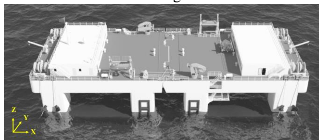
Fig.1. The connector of two semi-submersible floating platforms
