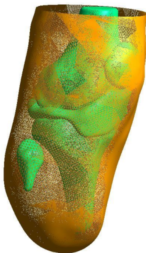
Figure 2: STL model of participants residual limb. Hard tissue surface is shown in green. Skin surface is shown in orange.
