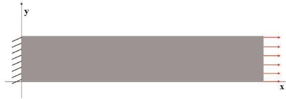
**Figure 8.** The loading and displacement boundary conditions of Case 2.
