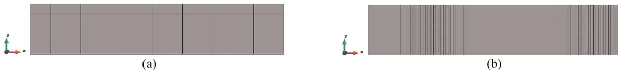
**Figure 9.** Two different meshes of Case 2. (a) 125 elements. (b) 2000 elements.
