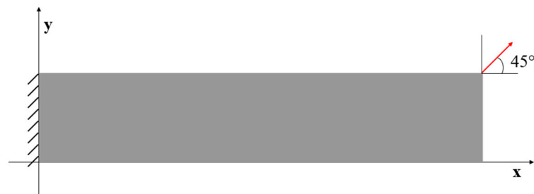
Figure 14. The loading and displacement boundary conditions of Case 3.
