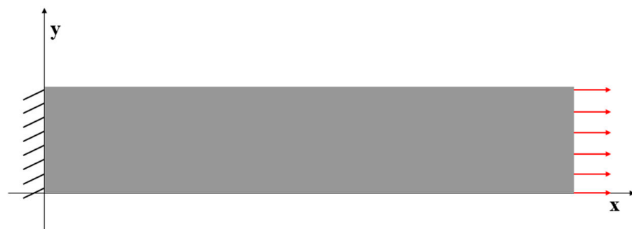
Figure 9. The loading and displacement boundary conditions of Case 2.
